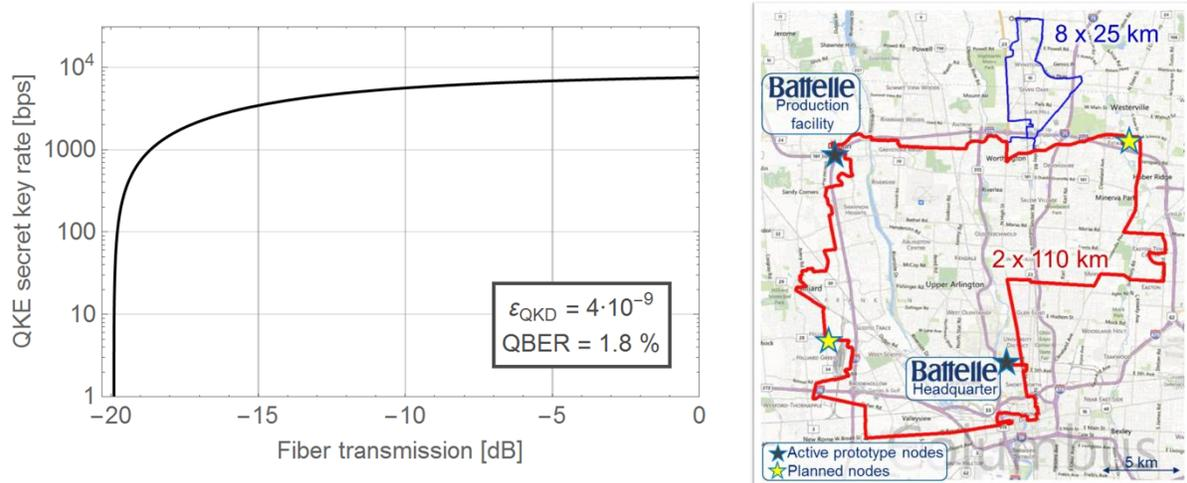
Figure 2. Left: Results of the design validation for the ATCA quantum blades based on a quantum key engine implementing the COW QKD protocol. Right: Layout of the Battelle QKD fiber network in the metropolitan area of Columbus (Ohio), which currently employs commercial QKD systems (Cerberis, idQuantique) to protect all communication between Battelle’s headquarters and its production facility in Dublin (Ohio).
