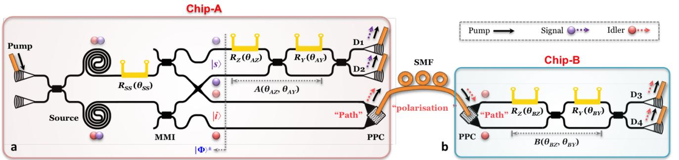
FIG. 2: **Quantum photonic interconnect and entanglement distribution between two integrated Si photonic chips.** a. Chip-A comprises path-entangled states generation, arbitrary projective measurement, and path-polarisation conversion (PPC). b. Chip-B includes a projective measurement and PPC. [10]
