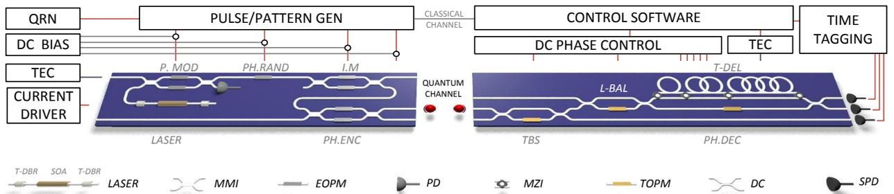
FIG. 1: **Integrated Photonic Devices for Quantum Key Distribution.** Schematic of the GHz clock rate, reconfigurable, multi-protocol, integrated indium phosphide transmitter device (left), which encodes quantum information with time-bin encoded, weak coherent light to be transmitted over optical fibre to a Silicon Oxynitride receiver circuit that passively decodes the quantum information with off-chip single photon detectors(right).
