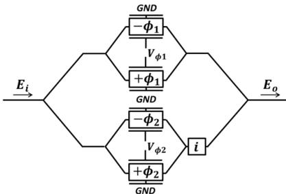
Figure1. The structure of DPM.
