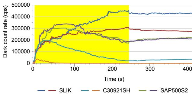
FIG. 2. Real-time recording of dark count rate before, during and after irradiation. Yellow shading denotes the time the radiation source was on. Sample temperature was  $0\text{ }^{\circ}\text{C}$ . The decrease of the count rate during irradiation in some of the samples occurred because the avalanche rate reached the peak saturation rate of the passively-quenched detector scheme, and overloaded it [8].
